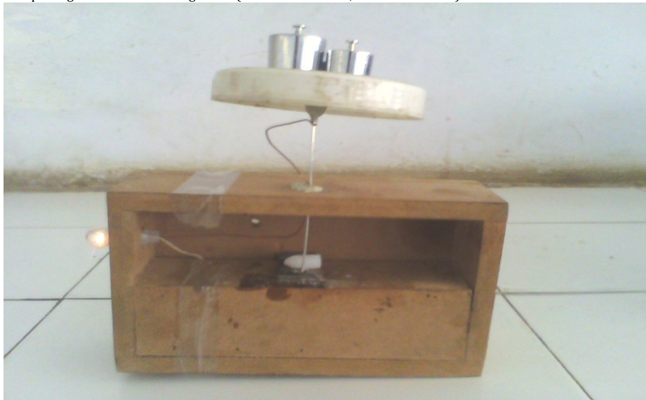
Figure 2. Breaking strength measurement of prepared suppository by Erweka tester.
