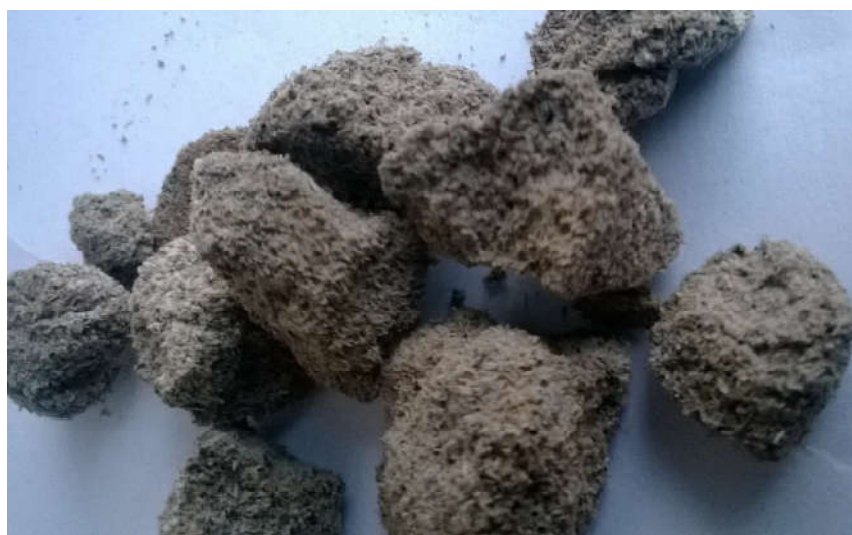
Figure 2: Picture of granules of silica gel immobilized sugarcane bagasse bio-sorbent
