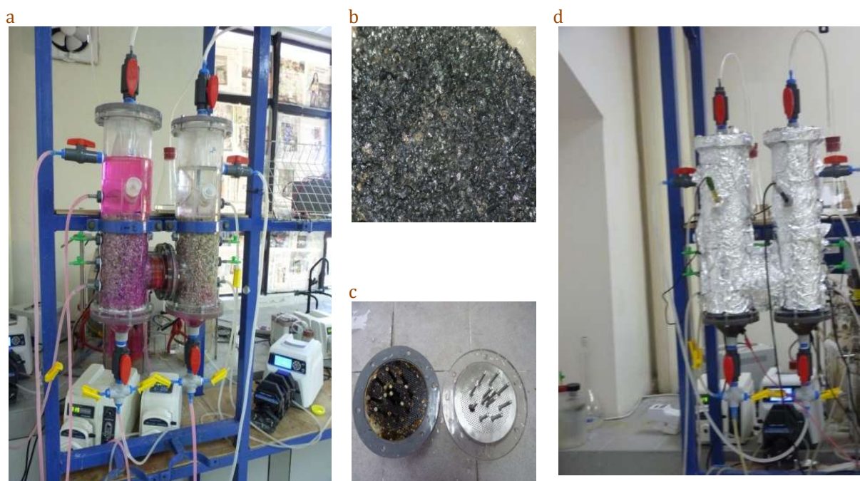
Fig. 1. Schematic of palm shell granular activated carbon twin chamber up-flow reactor (PSGAC-TCUR), when the carrier is sand (a), and GAC (b), stainless steel as electrode and flow distributor (c), and when the reactor runs as BER and carrier is GAC
