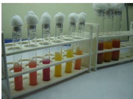
Fig 5: Positive MPN tubes showing Acid gas production
